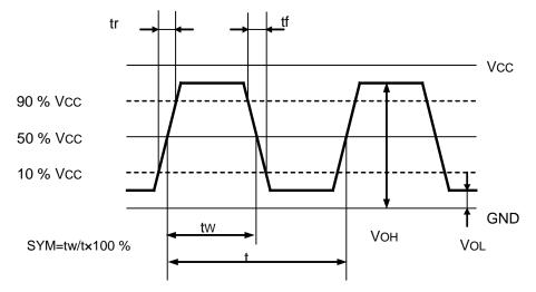
4-2) Output waveform (Clipped sine wave output)
