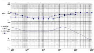
2-14) MTIE (19.2MHz, Loop BW=0.1Hz) Constant temperature : +25 deg.C
