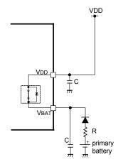
[Connection example when not using the battery backup switchover function]
