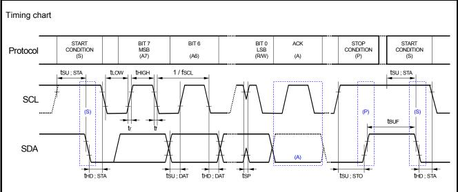
When accessing this device, all communication from transmitting the start condition to transmitting the stop Caution: condition after access should be completed within 0.95 seconds. If such communication requires **0.95 seconds** or longer, the I<sup>2</sup>C bus interface is reset by the internal bus timeout function.
