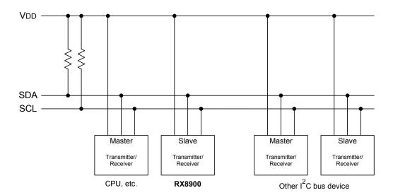
Any device that controls the data transmission and data reception is defined as a "Master".
