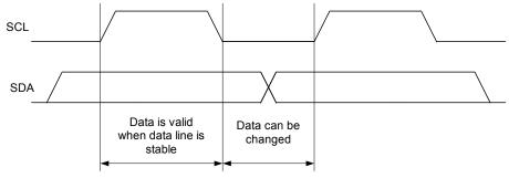
\* Note with caution that if the SDA data is changed while the SCL line is at high level, it will be treated as a START, RESTART, or STOP condition.
