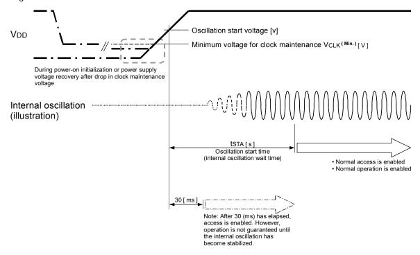
3) When the read VLF-bit value is "VLF = 0 (normal status)", access is enabled without waiting for stabilization of oscillation.
